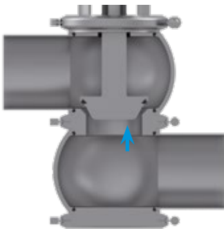
Control valve with linear control cone
