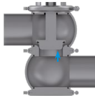
Control valve with equal-percentage control cone
