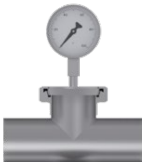
Formation of a dome by conventional adaptation at the T-piece
